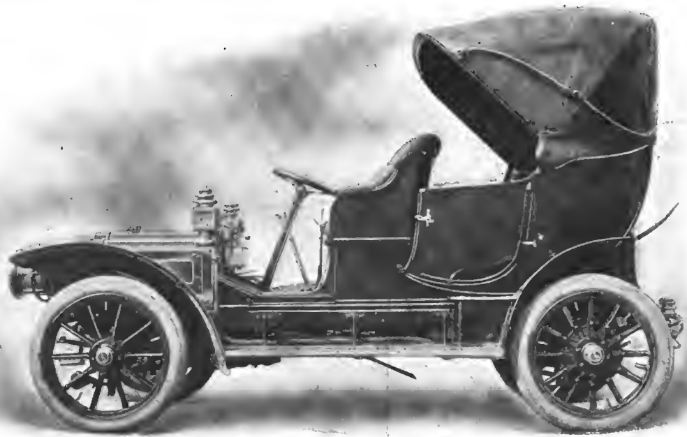
AMERICAN MORS TOURING CAR, 4 CYLINDERS, 14-18-H.P., PRICE $3,000. St. Louis Car Co., St. Louis, Mo.
